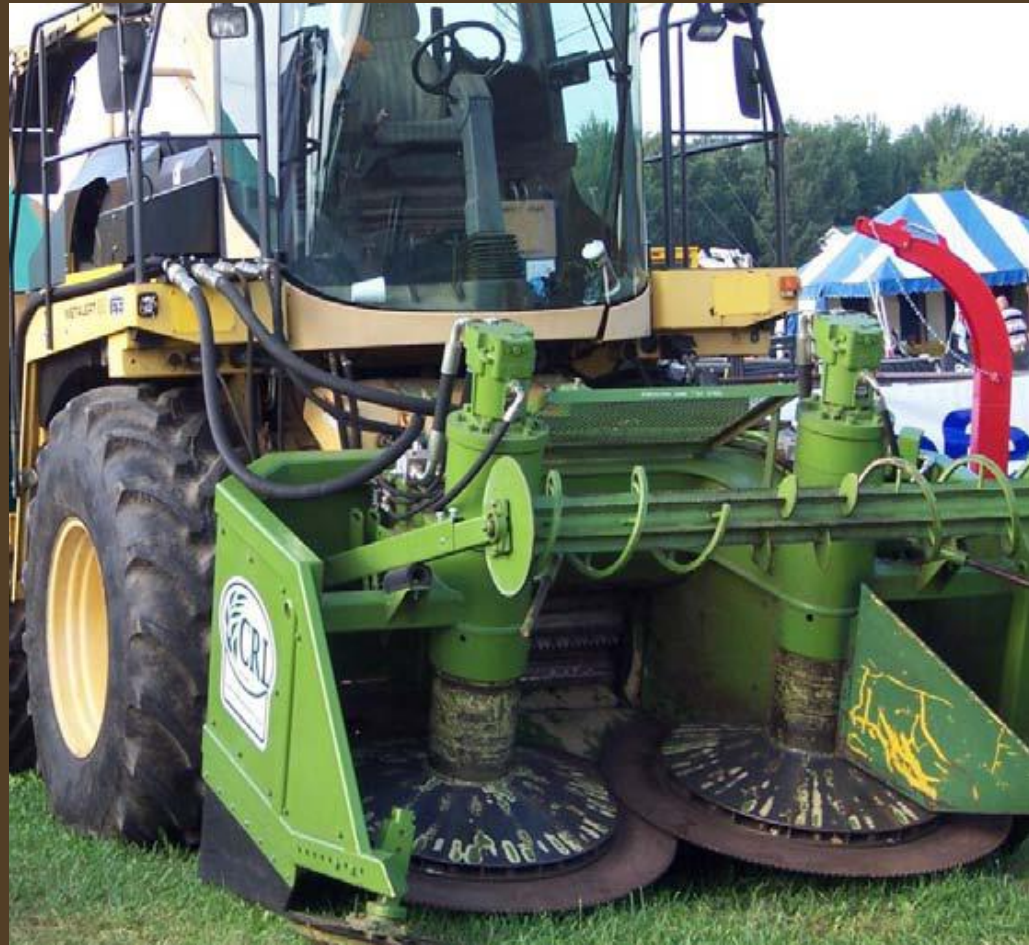
Coppice Resource Limited header to fit CASE NEW HOLLAND FX SERIES forage harvester
